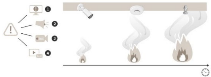
Fire detection based on video reacts faster than traditional smoke detectors.
